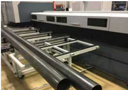
Tubes up to 6 m of length are removed by automatic unloading system with conveyor.
