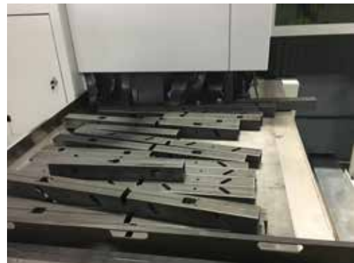
Tubes up to 6 m of length are removed by automatic unloading system with conveyor.
